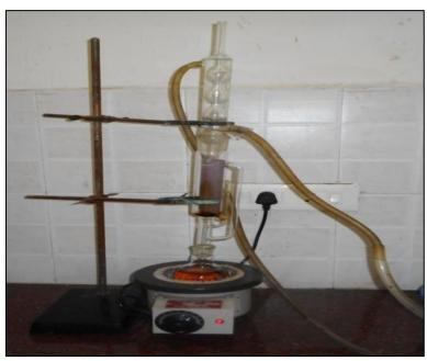
Materials Required: Turmeric powder (Curcuma longa), Soxhlet apparatus Round bottom flask, Heating mantle or water bath, Condenser, Filter paper or thimble, Organic solvent (commonly used: ethanol, methanol, or acetone), Weighing balance Beaker, funnel, and glassware.
