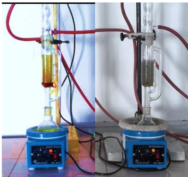
Figure 2. Extraction of Flaxseed Components by using Soxhlet Extractor.
