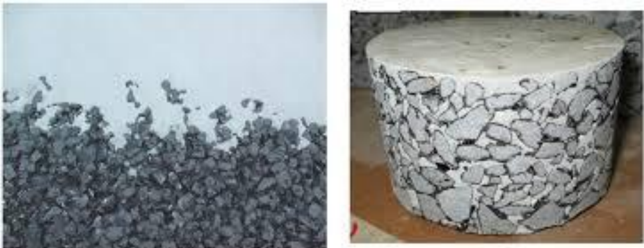
Fig. 2. Penetration of grout of trial 5.
