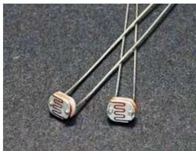
Fig 2. Light Dependent Resistor (LDR)
