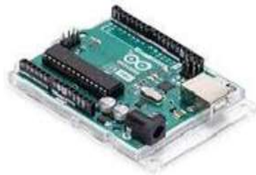
Fig 1. Arduino Uno microcontroller board.
