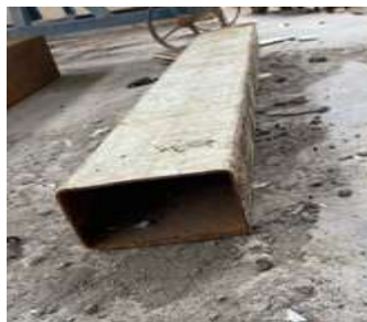
Figure 2.3 Steel hollow section
