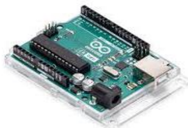
Fig 2. Arduino Uno microcontroller board.
