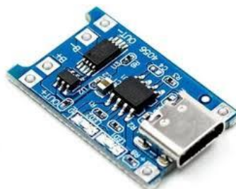
Fig. 6. BQ001A battery charging module.
