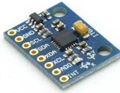
Fig 3. MPU6050 inertial measurement unit (IMU).
