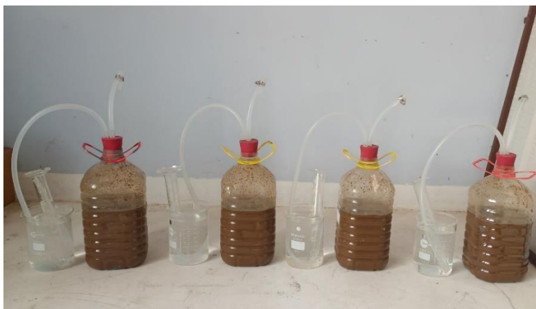
Fig 3: laboratory setup for the anaerobic digestion (different ratio)
