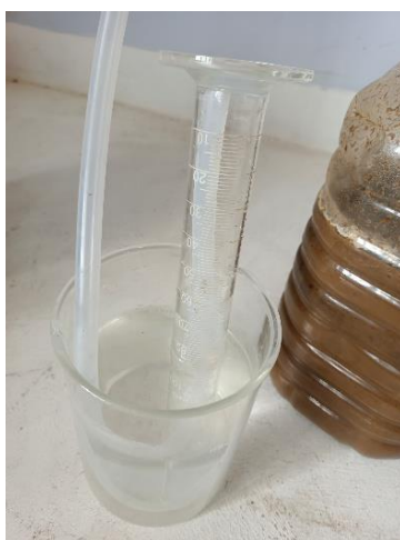
Fig 2: setup for gas displacement measurement
