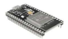
The ESP32 module is used in solar wireless electric vehicle charging systems to monitor the charging process, collect data, and provide real-timefeedback to the user. It monitors the charging process in real-time. It collects data about the charging process. It provides feedback to the user in real-time. It helps make the charging stationefficient and reliable.
