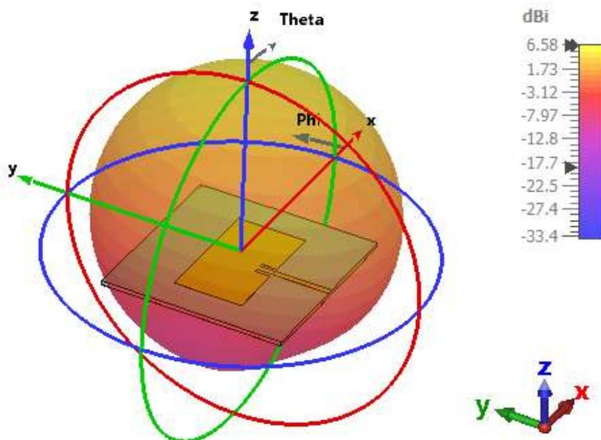
Fig 7. 3D model of a RPMA with color-coded gain
