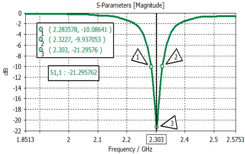
Fig. 4. Simulation of Return loss against frequency.
