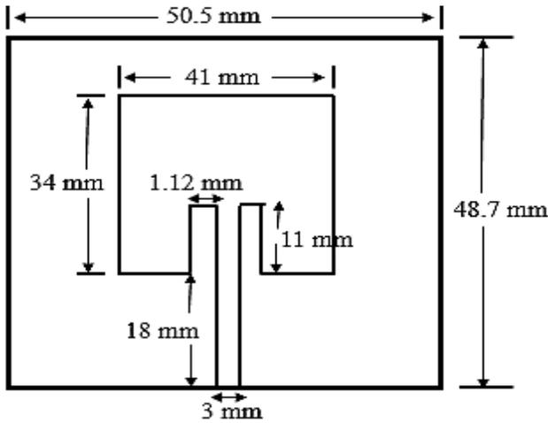
Fig. 1. Design of Microstrip patch Antenna (Theoretical)
