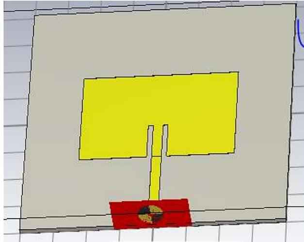
Fig. 2. The proposed RMPA modelled in CST.
