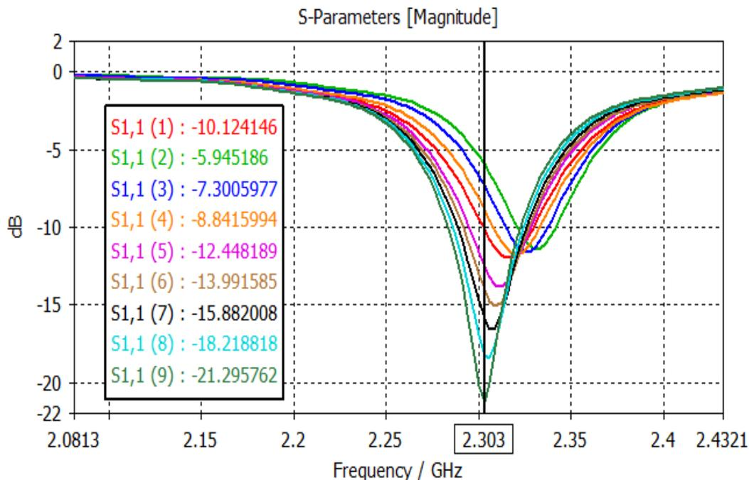
Fig. 3. Graph of Return loss of gap inset feed against frequency
