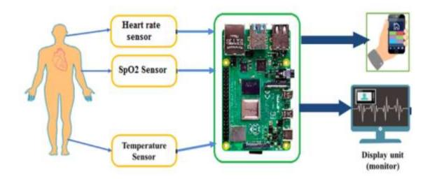
• Data Flow: Data is collected via sensors, transmitted to the Raspberry Pi, and then processed. The results are displayed and stored for long-term analysis. The system architecture ensures minimal latency to facilitate near-instantaneous alerts.
