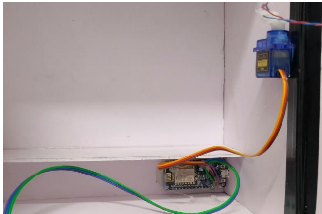
Fig g. Circuit with Servo Motor for Locker Mechanism
