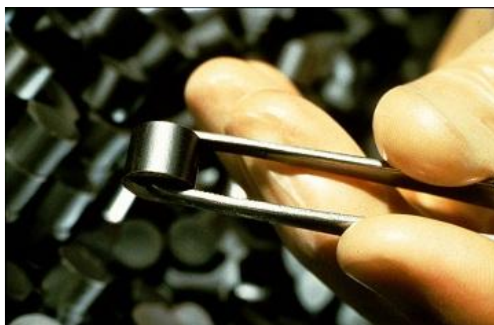
Figure 15. An enriched nuclear fuel pellet (Wikimedia Commons. (June 17, 2015). Fuel Pellet
