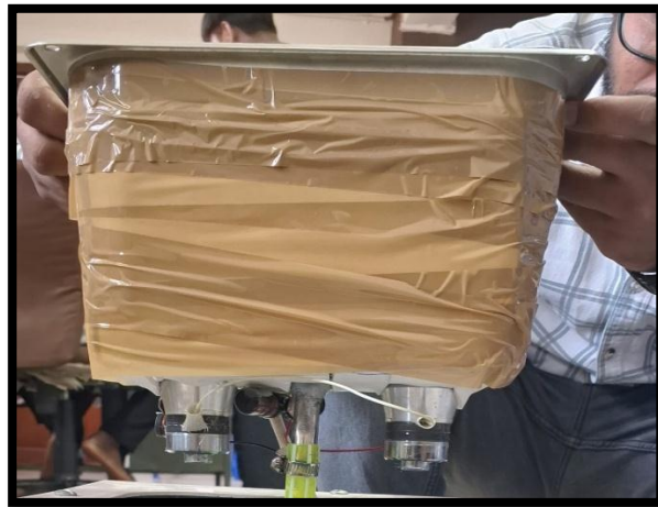
Fig. Picture of Transducer & Insulation
