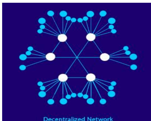
Fig shows the Resource sharing structure of Decentralised network which has no single authority server controlling the nodes, all the nodes works independently as individual.
