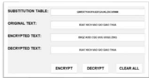
Fig.2. Results of Encoding and Decoding Using the Custom 26-Letter Character Substitution Table (e.g., QWERTYUIOPASDFGHJKLZXCVBNM)
