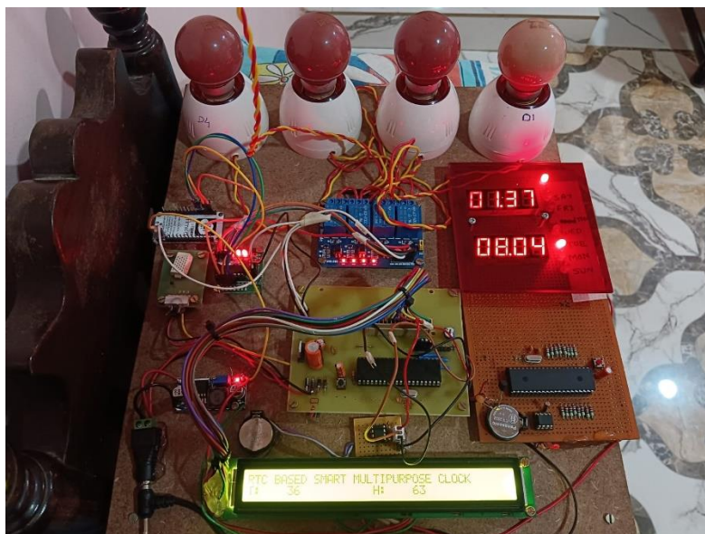
Fig. 3.A) Implementation of Digital Clock
