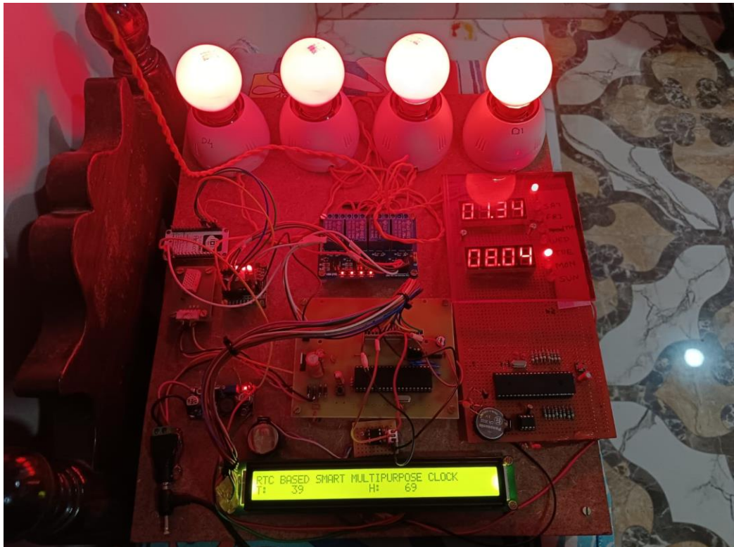
Fig. 3.B) Implementation of Reminder and Home Automation System
