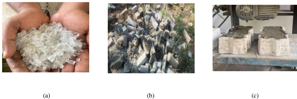
Fig. 1 - (a) pet flakes; (b) C&D waste as aggregate; (c) casting paver blocks
