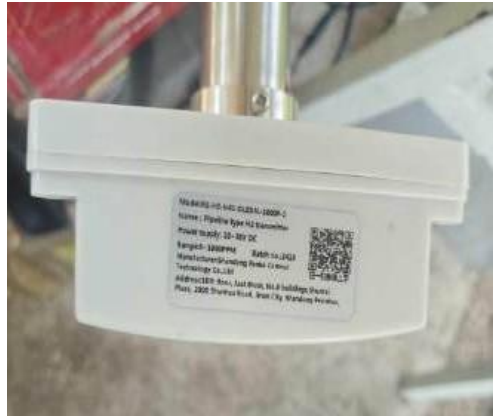
Figure 10.1 RS-H2-N01-OLEDL-1000P-2 (Gas Sensor for Hydrogen gas)
