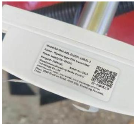
Figure 10.2. RS-CH4-N01-OLEDL- 100LEL-2 (Gas Sensor for Methane)
