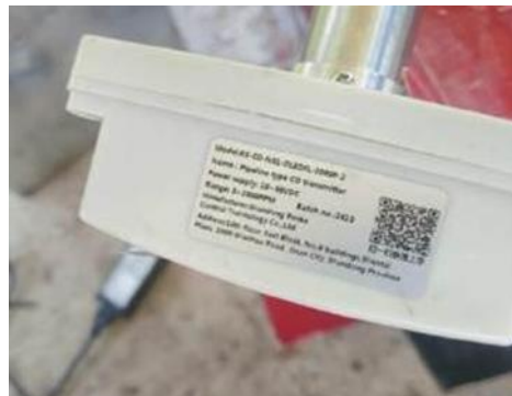
Figure 10.3. RS-CO-N01-OLEDL- 2000P-2 (Gas Sensor for Carbon Monoxide)
