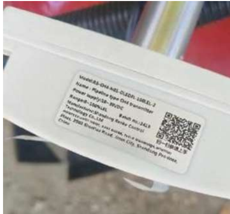
Figure 10.2. RS-CH4-N01-OLEDFL- 100LEL-2 (Gas Sensor for Methane)
