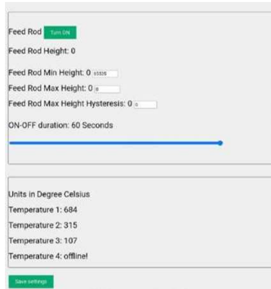
Figure 7.2. Screenshot of the Web Interface Settings (Feed Rod Height and Temperature)
