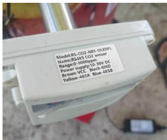
Figure 10.4. RS-CO2-N01-OLEDL (Gas Sensor for Carbon Dioxide)
