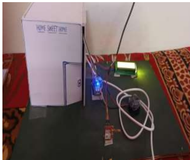
Figure 2. Model Of Theft Detection system Using PIR Sensor
