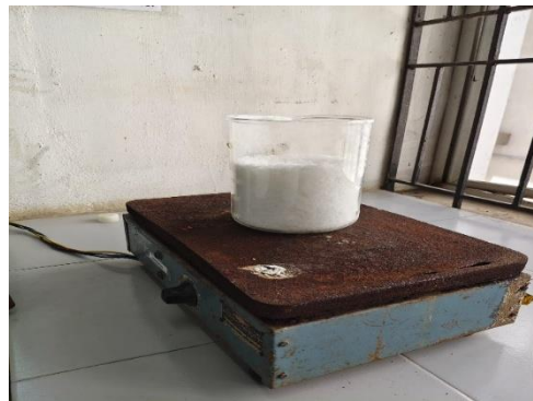
Fig.5 Heating the PCM on Hot Plate
