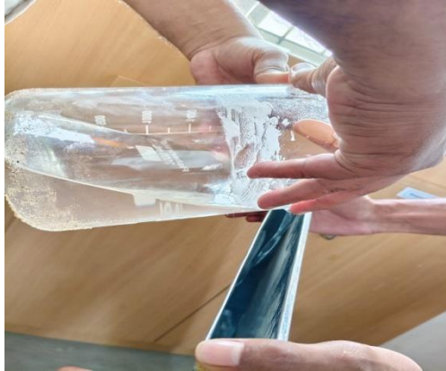
Fig.7 Poured the melted PCM into Storage box
