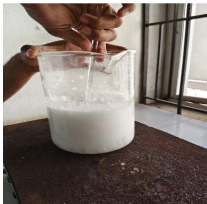
Fig.6 Stirring the PCM with Glass Rod
