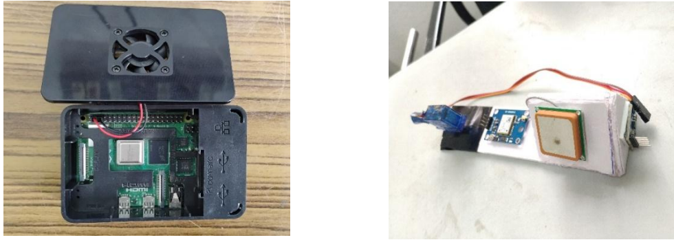
Fig. 2 – (a) Raspberry Pi 4 Model B; (b) Navigation Setup.
