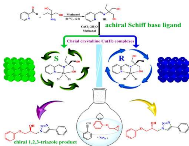
Fig. 1 - Asymmetric Synthesis of Chiral 1,2,3-Triazole Products Using Chiral Cu(II) Complexes [11].
