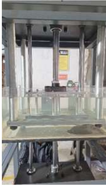
Figure 12 :- Actual Testing and Validation of fixture using Leakage testing Machine
