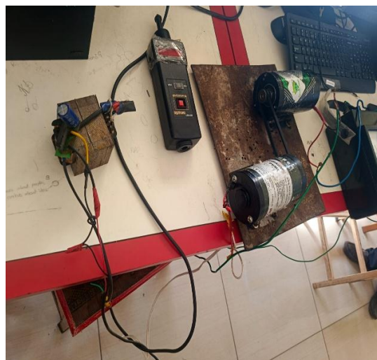
Figure 2. Dual rotor generator with connections
