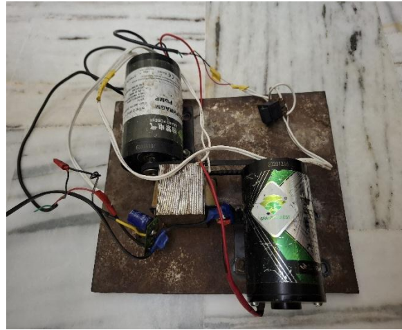
Figure 1. Dual Rotor Generator
