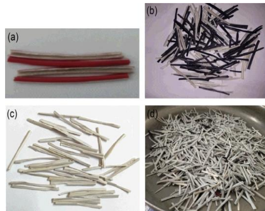
Fig.2. PVC fibers from e-waste used in concrete
