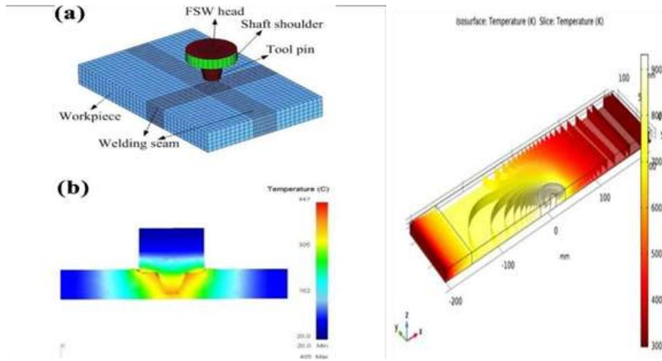
Fig 5:- Visualizations of FEM simulation results showing temperature distribution and material flow for various tool pin profiles.
