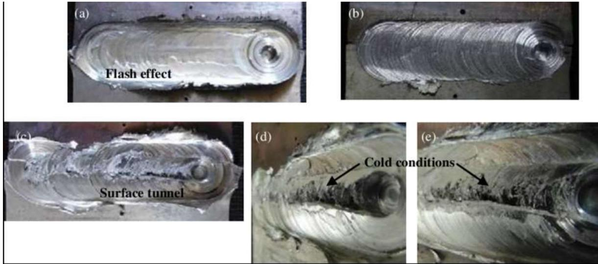
Fig-8:- Photographs showing the appearance of defects such as voids and cracks in welds with cylindrical, tapered cylindrical, square, triangular, and hexagonal tool pin profiles.
