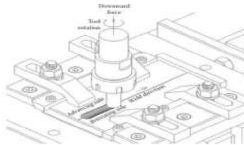
Figure 2. Schematic of FSW process
