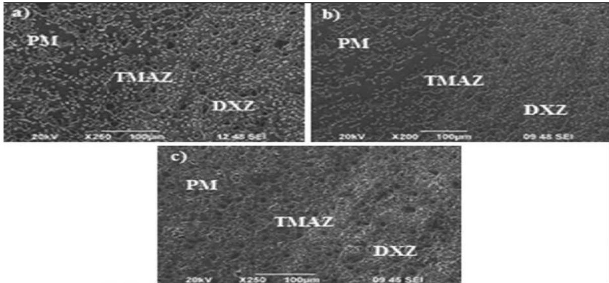
**Fig-7** High-resolution images of the HAZ, TMAZ, and stir zone (SZ) showing the microstructural variations based on cylindrical, tapered cylindrical, square, triangular, and hexagonal tool profile.
