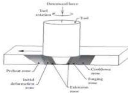
Figure 1. Stages in the Friction Stir Welding (FSW) process
