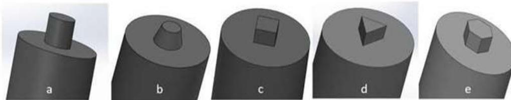
Figure 3 FSW tools with different pin profile (a) cylindrical; (b) tapered cylindrical; (c) triangular; (d) square and (e) hexagonal.
