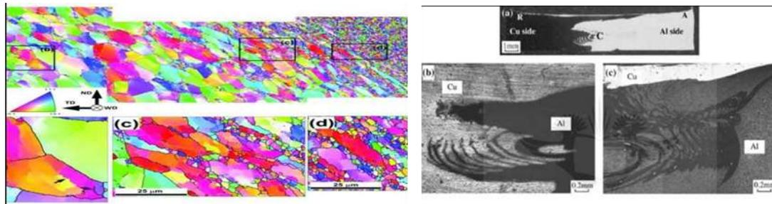
Fig 6:- Comparative microstructure images showing the grain refinement effects from cylindrical, tapered cylindrical, square, triangular, and hexagonal tool profiles.:
