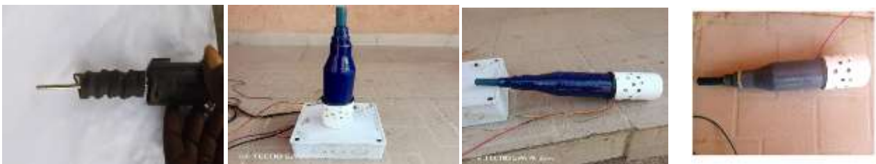
Plate 2: showing dc motor connected to the impeller
