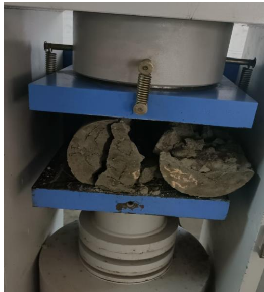
Fig -4: split tensile test on cylinder
