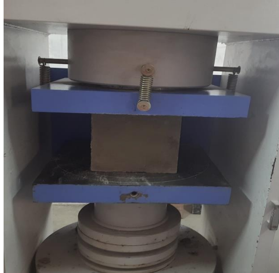
Fig -3: Compressive test on cube
