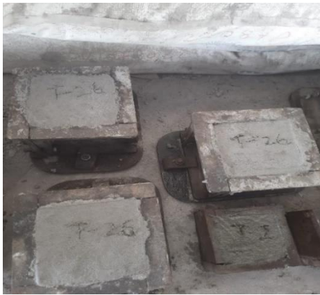
Fig 3 a. Casting of cubes
