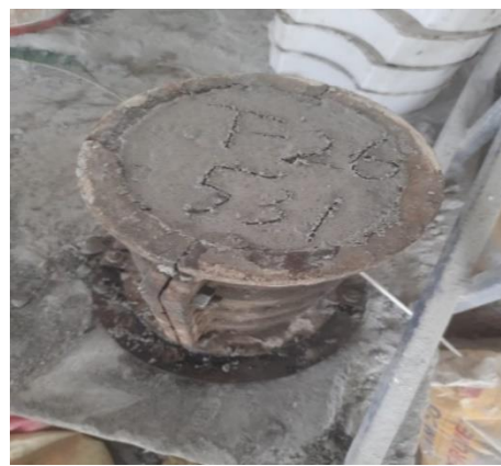
Fig 4 b. Casting of cylinders
