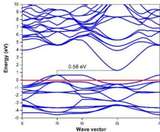
Figure 3: Band structure of CsAgI<sub>3</sub> calculated using PBE with ultrasoft pseudopotential, represented for the energy of -5 to +10 eV.
