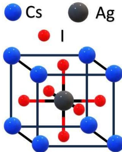
Figure 1: Cubic perovskite structure of  $\text{CsAgI}_3$  related to the pm-3m space group. Where Cs is at (0,0,0), Ag is at (0.5, 0.5, 0.5),  $I_1$  is at (0, 0.5, 0.5),  $I_2$  is at (0.5, 0, 0.5) and  $I_3$  is at (0.5, 0.5, 0) positions.
