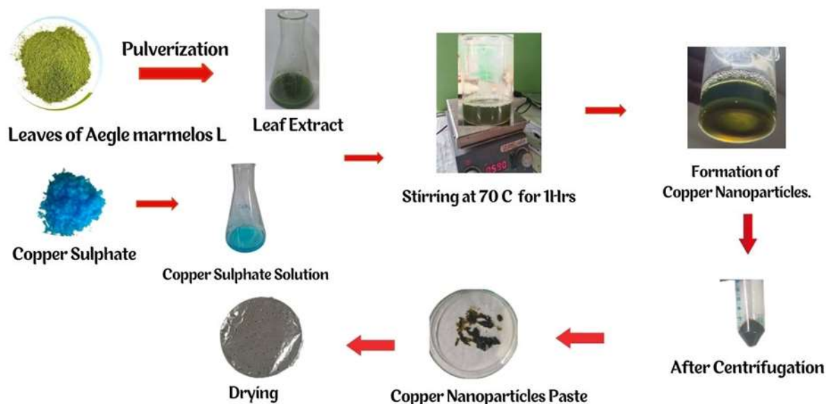
Figure 1: Schematic Diagram showing the synthesis of Copper sulphate Nanoparticles from Aegle marmelos L Aqueous extract.
