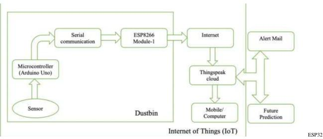
NodeMCU: Acts as the central controller, processing sensor data and transmitting information via WiFi.
