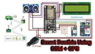
Trigger Pin (TRIG)  $\rightarrow$  GPIO 5
