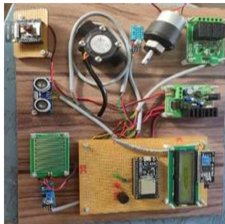
Figure 3: Hardware of IOT Based Flood Detection and Alerting System Using Decision Tree Algorithm
