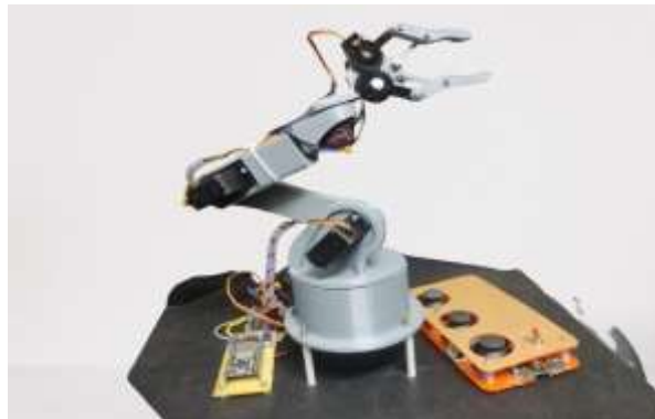
Figure3:Hardware of Wireless Joystick Control Robotic Arm Using ESP32 Microcontroller
