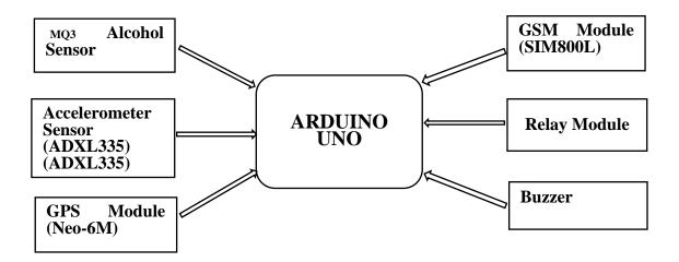
The Smart Helmet System works on the principle of sensor-based safety enforcement and IoT-enabled accident detection and alert system. The system consists of various sensors and electronic components integrated into the helmet and the bike unit to ensure the rider's safety. It incorporates features such as helmet detection, alcohol detection, accident detection, and emergency alerts.
