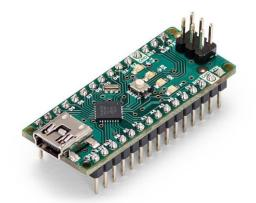
The Arduino Nano serves as the central controller, executing the firmware that manages motion control, laser intensity, and engraving patterns. It communicates with all components to synchronize their operation based on user input or pre-loaded engraving instructions.
