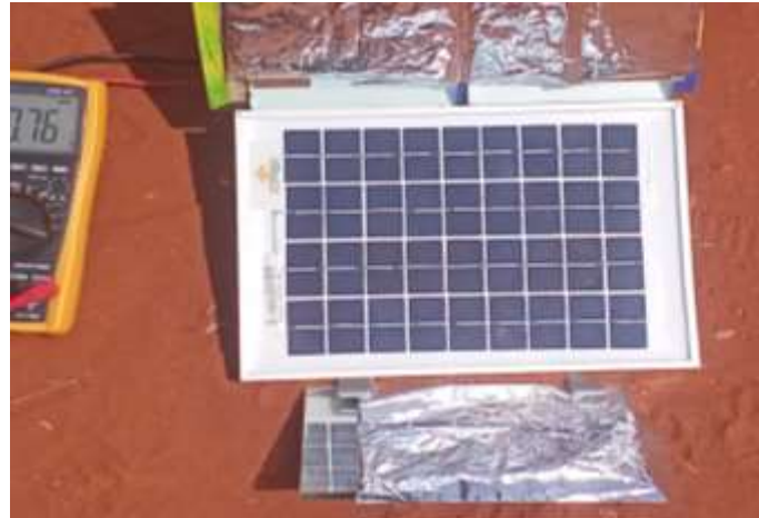
Figure 10. Voltage reading for PV panel with mirror & aluminium foil
