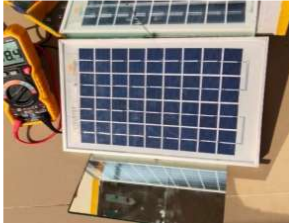
Figure 7. Amperes reading for PV panel with mirror
