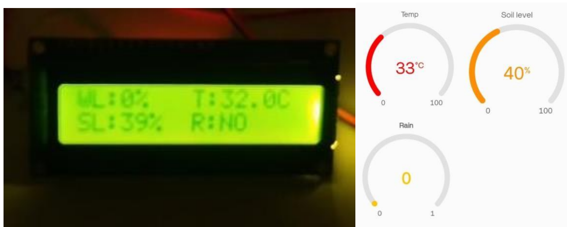
Fig. 4.2 Output of Soil Moisture, Temperature, and Rain Alert
