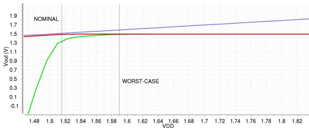
Figure 3: Input voltage sweep - dropout and regulation region
