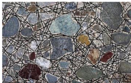
Figure 2. Steel fiber distribution in concrete mixes (Source: Journal Of Steel Fiber Reinforced Concrete Behaviour, Modelling And Design, 2017)
