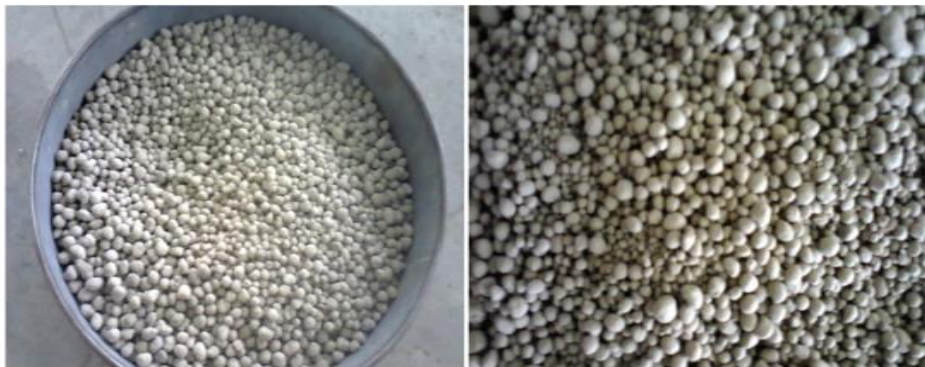
Figure 2. Pelletized aggregates obtained from the pelletizer
