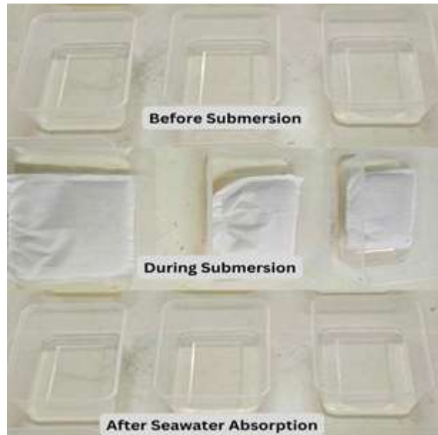
Figure 14. Pad Submersion Process for Setup 2 Before, During, and After
