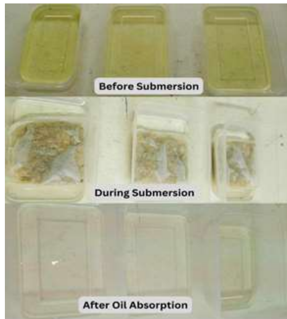
Figure 13. Pad Submersion Process for Setup 1 Before, During, and After
