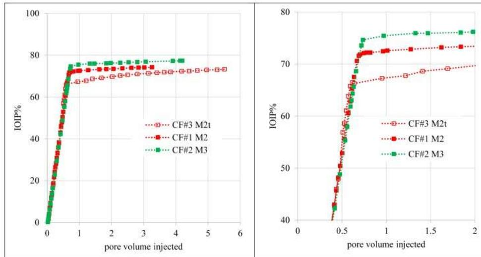
Figure 4 graph showing oil recovery for a long time of injecting water with a high salinity
