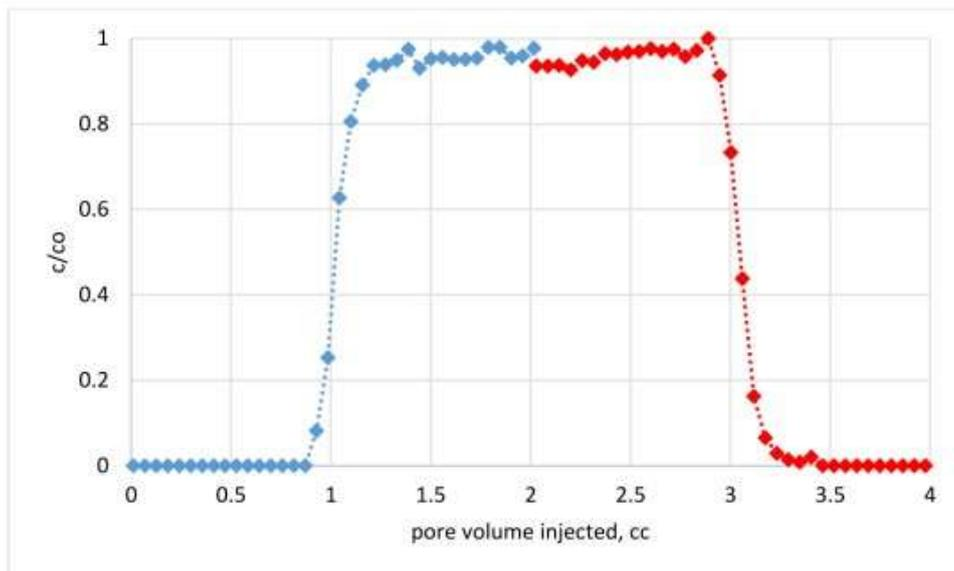
Figure 6: The results of the core homogeneity test on the lithium concentration profile (normalized to the initial lithium concentration)
