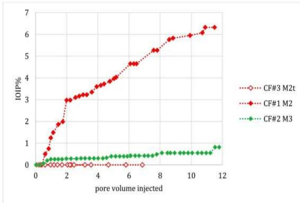
Figure 7: Recovering Oil While Injecting Low-Salinity Water
