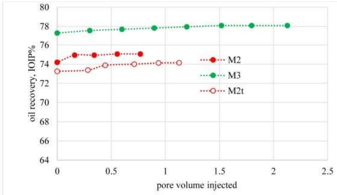
Figure 5 :0 PV in this graph shows the end of the primary flow rate (4 cc/hr) during a flood powered by high salinity water injection.
