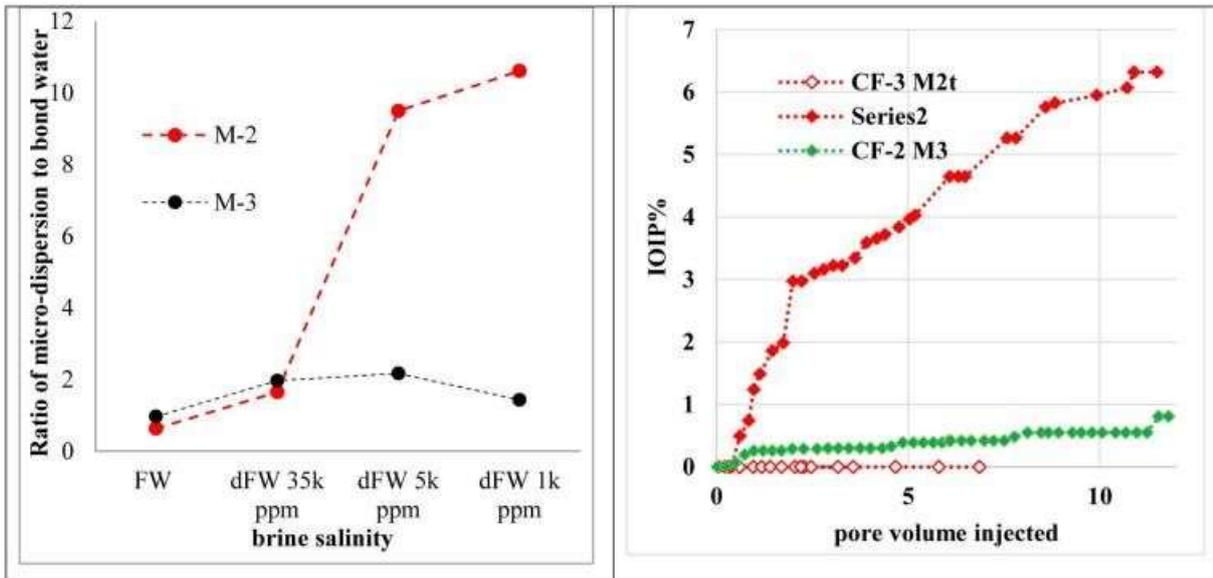
Figure 10—Left plot displays Crude-M2 and Crude-M3 micro-dispersion data. The right-hand plot shows tertiary LSWI's increased oil recovery. CF#3 uses Crude-M2t.
