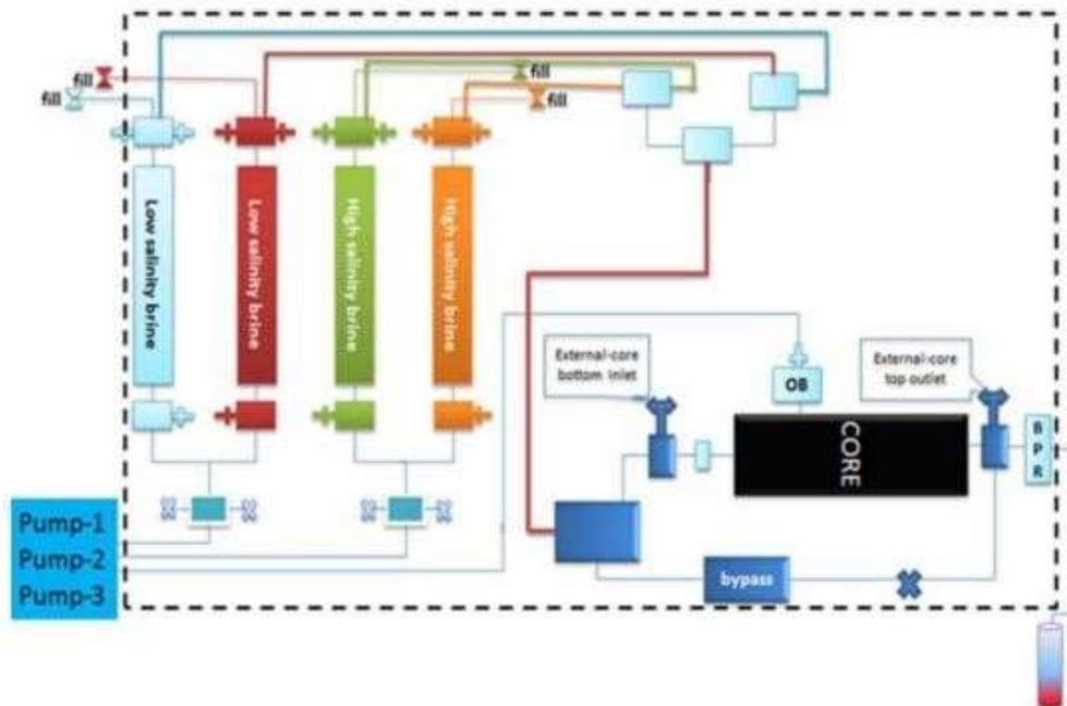
Figure 3. diagram of coreflood rig
