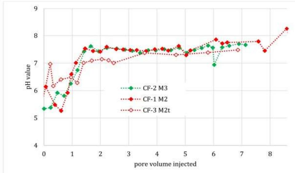
Figure 8: When low-salinity tertiary water is injected into a core test, the pH of the effluent water changes.
