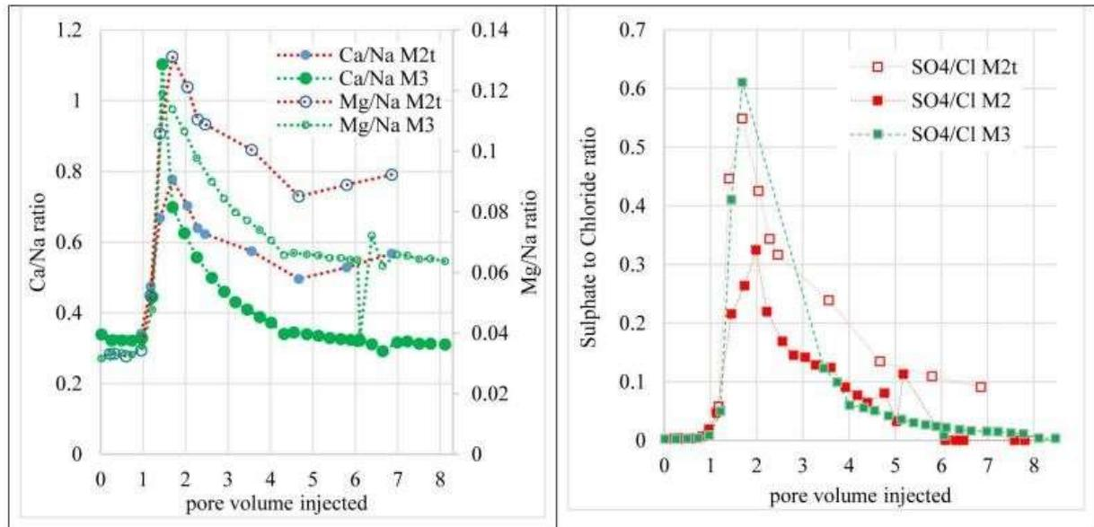
Figure 9: Changes in Ca and Mg concentrations during tertiary low salinity water injection are seen on the left plot. Figure depicting effluent SO<sub>4</sub>/Cl shift during tertiary low salinity water injection is accurate.
