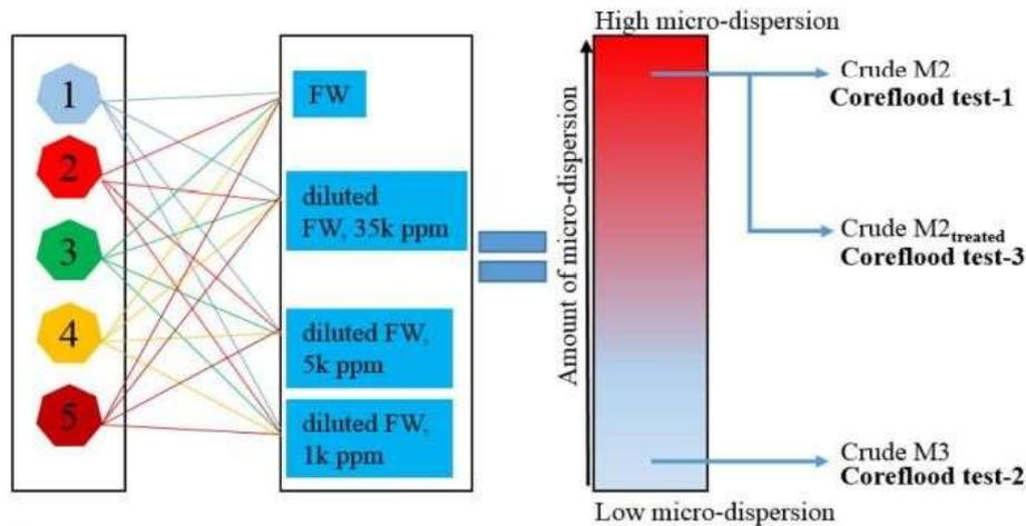
Figure 1: Test design for detecting water microdispersion in crude oils at varying salt concentrations Microdispersion testing of crude oils at varying salt concentrations
