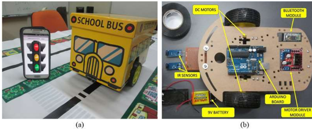
Fig. 2 Line-follower robot; a. Traffic light app; b. Robot design
