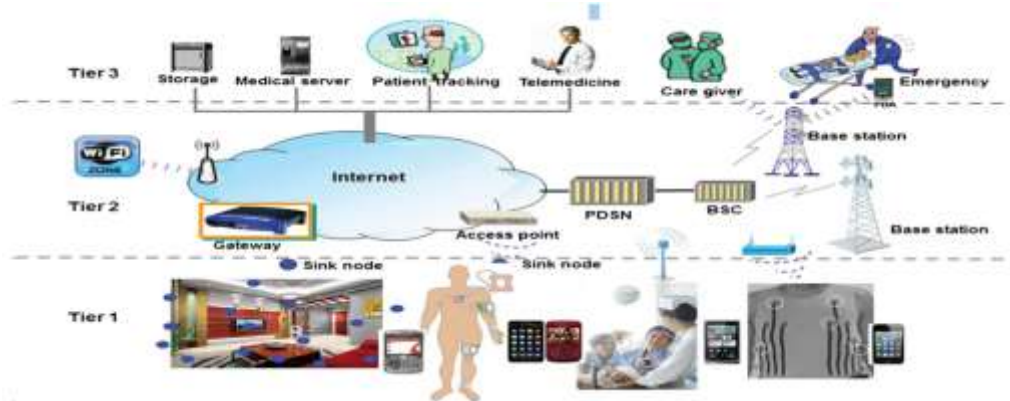
Fig. 6: Three-tiered architecture for WSNs in healthcare
