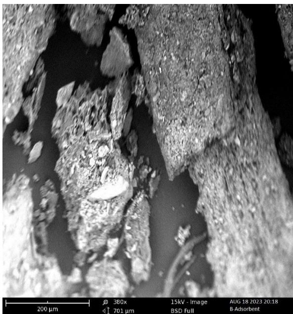
Figure 5: SEM image of n-Hexane neem leaf extract mediated ZnO NPs at 380x magnification
