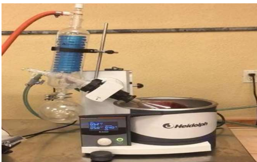
Figure no.7. Solvent recovery by rotatory evaporator
