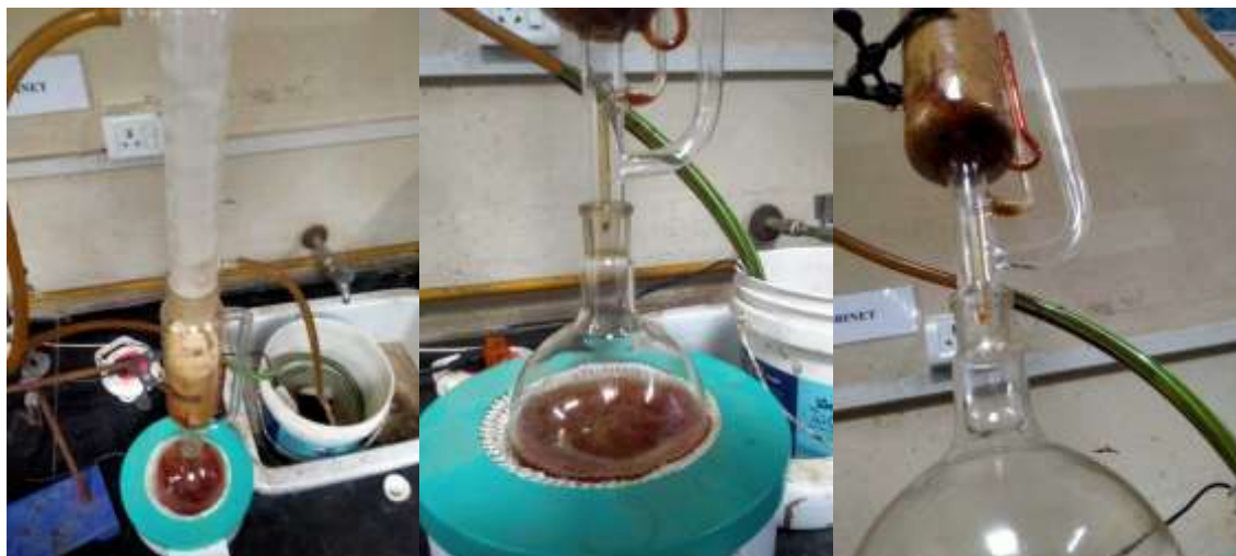
Figure no.6. Soxhlet extraction process
