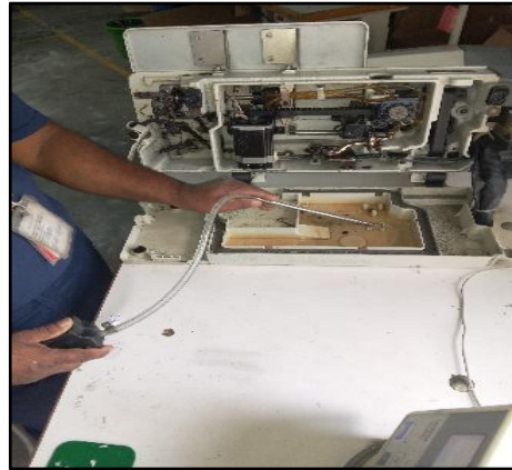
(Figure 5- Oil service Operation)
