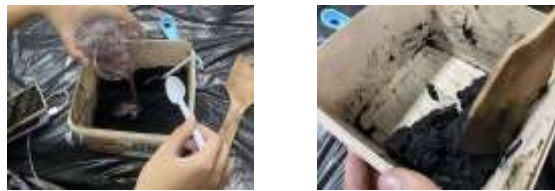
Image 8 & 9: Mixing of jackfruit peel powder and taro root mucilage.
