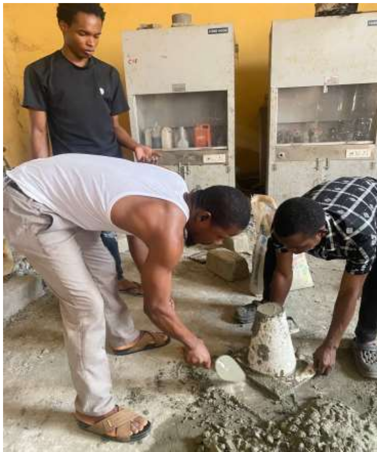
Fig 3: concrete mix slump test
