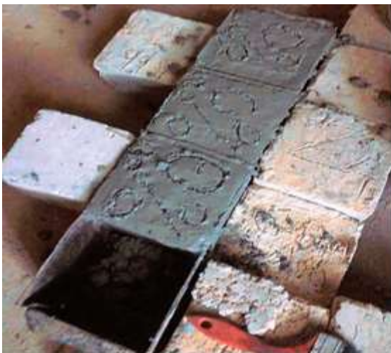
Fig. 5: Freshly mixed concrete cast in cube moulds
