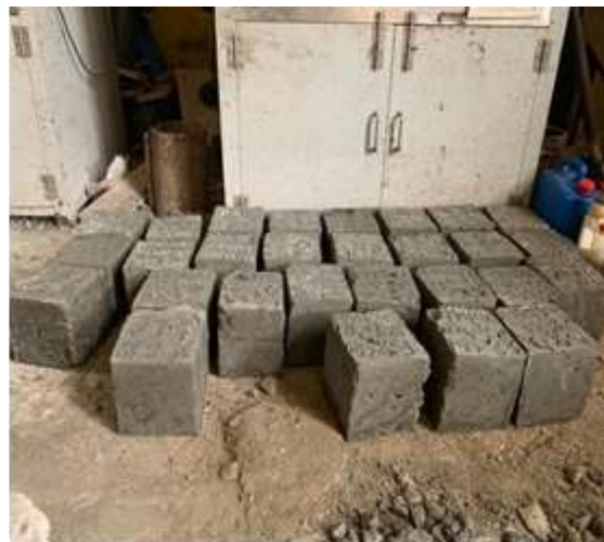
Fig. 6: Demoulded concrete cube moulds
